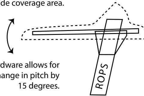
Hardware allows for change in pitch by 15 degrees.
