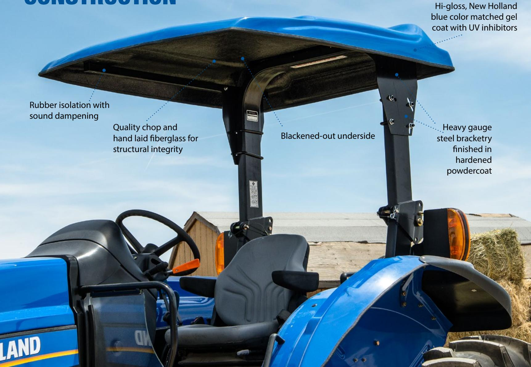
Rubber isolation with sound dampening
